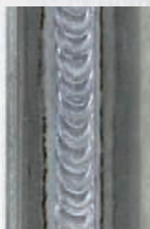
Aluminium superPuls PF Position
